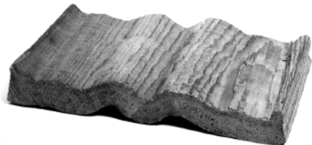
Figure 12-10. Severe collapse in western redcedar.
